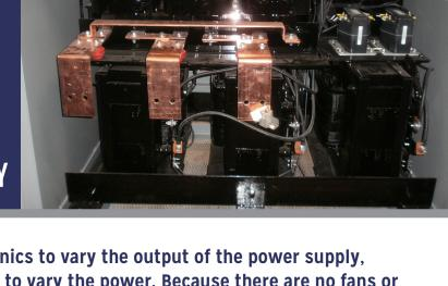
Instead of using solid state electronics to vary the output of the power supply, these units use a saturable reactor to vary the power. Because there are no fans or solid-state devices, saturable reactors can operate in environments that would be harmful to silicon controlled rectifier power supplies due to high temperatures or unclean conditions. Magnetic Specialties design saturable reactors to fit existing control schemes.
