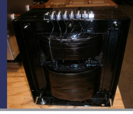
Ferroresonant Transformers are also known as Constant-Voltage Transformers (CVT). A CVT regulates its secondary voltage typically within a few percent even when the primary voltage changes as much as 15-20 percent. Accompanying these transformers is a bank of capacitors. These capacitors are used to tune the output voltage of the CVT and are essential to its proper operation.
