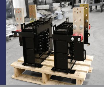
DC choke reactors are a type of inductor used on the output of a rectifier to filter or "choke" any high frequency AC component superimposed on the DC. The impedance of an inductor increases with frequency, allowing the low frequency DC to pass while blocking the higher frequency AC signals.
