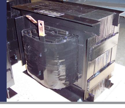
A Current Limiting Reactor (CLR) is commonly used in the primary circuit of an electrostatic precipitator's TR set. Electrostatic precipitators are used for pollution control in paper mills, power plants, and even restaurants. Magnetic Specialties can design and manufacture single and multi-tap CLRs for a variety of line frequencies including 400 Hz operation.
