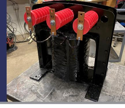
Control transformers are used to step down supply voltages to a lower, safer voltage for control circuits and other low power devices, such as relays, contactors, motor starters, and signaling devices.
