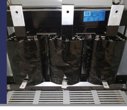
Auto transformers have one winding which acts as the primary and secondary. As a result, when compared to a traditional transformer of equivalent KVA rating, an auto transformer will be smaller and lighter. For voltage ratios that do not exceed about 3:1, an autotransformer is typically a less expensive option then an isolation transformer. If isolation between input and output is not a requirement for your application, a MSI auto transformer is an excellent choice.
